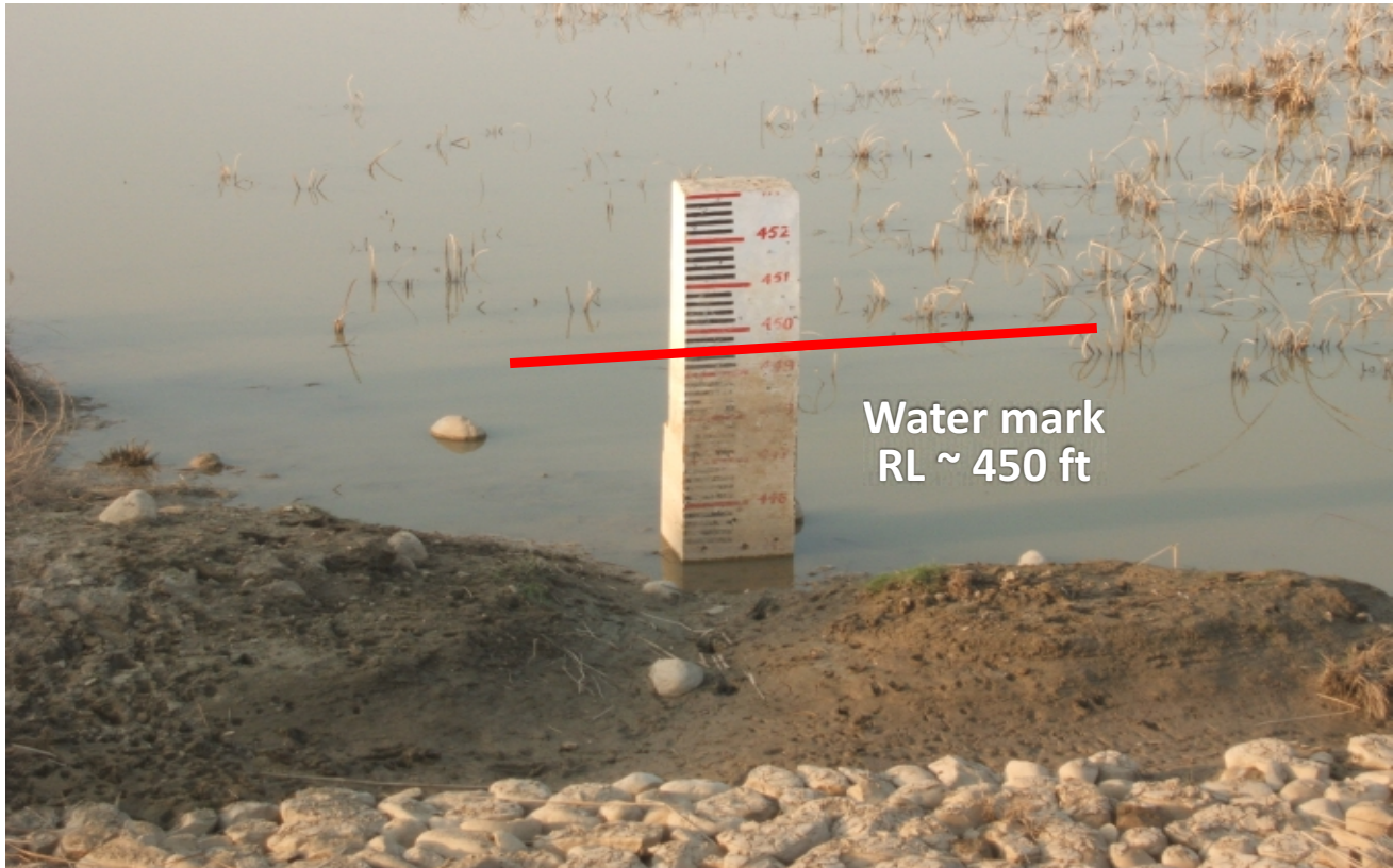
Photo showing water mark on a gauge area between Spur # 2-A and Shank of Spur # 2
