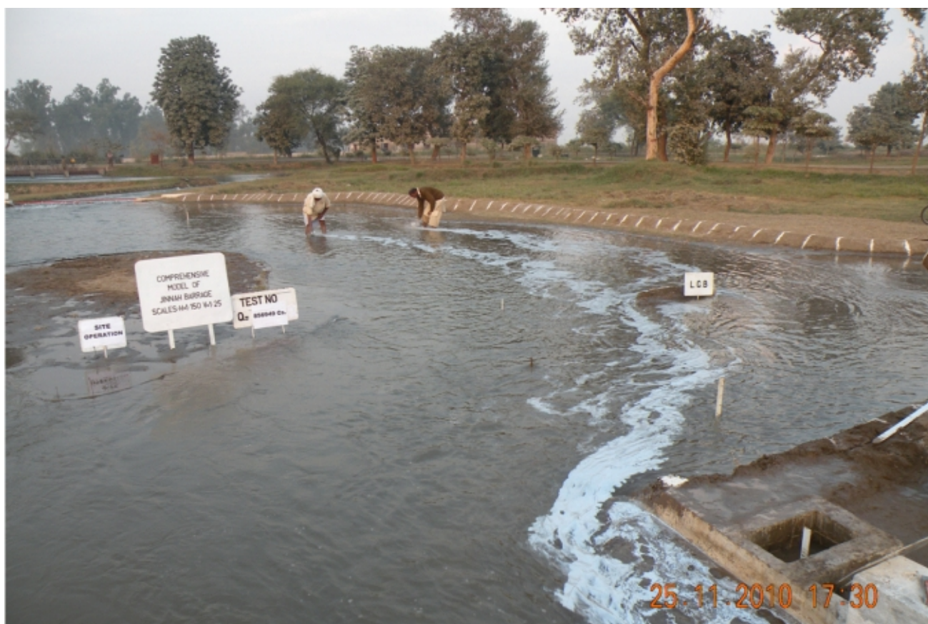
Site Operation of Barrage at Q = 8,56,949 Cusec
