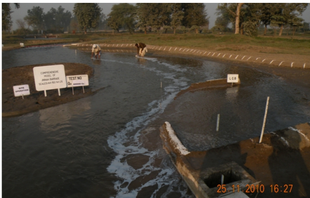
Site Operation of Barrage at Q = 6,00,000 Cusec
