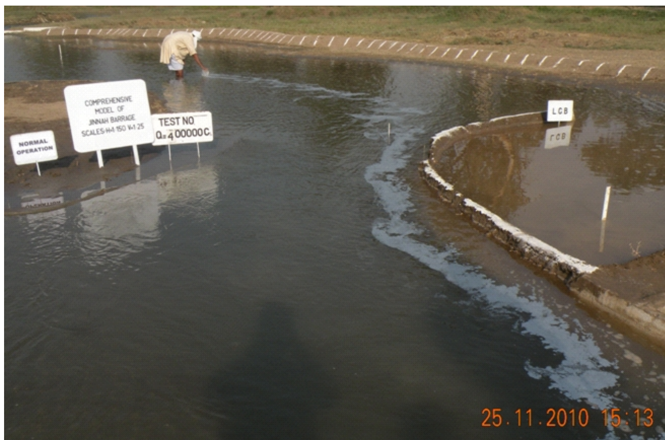
Normal Operation of Barrage at Q = 4,00,000 Cusec
