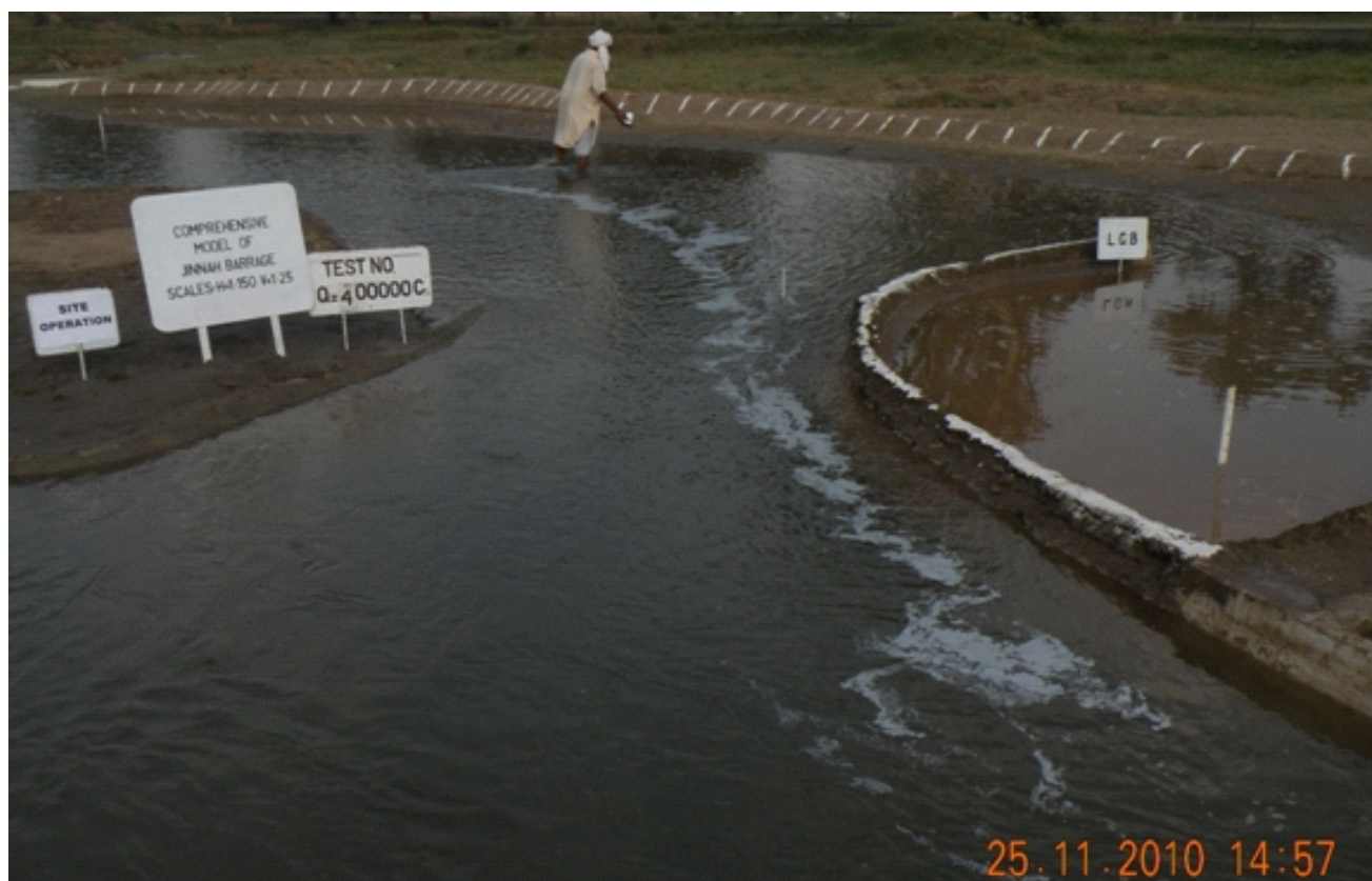
Site Operation of Barrage at Q = 4,00,000 Cusec
