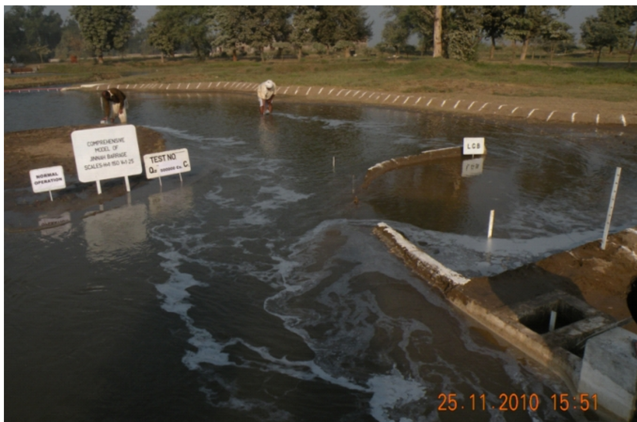
Normal Operation of Barrage at Q = 5,00,000 Cusec
