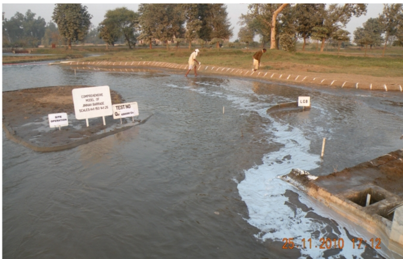
Site Operation of Barrage at Q = 6,60,000 Cusec
