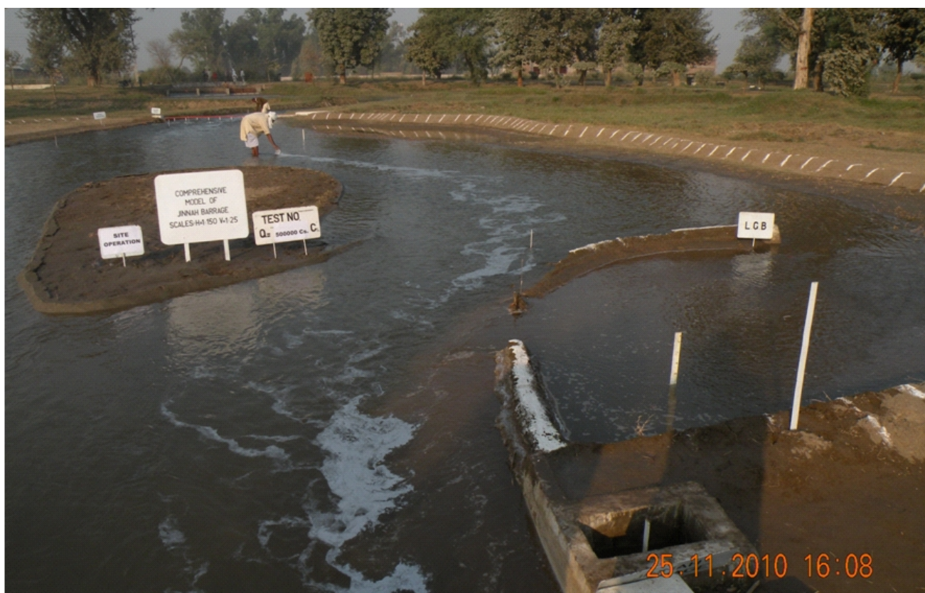
Site Operation of Barrage at Q = 5,00,000 Cusec
