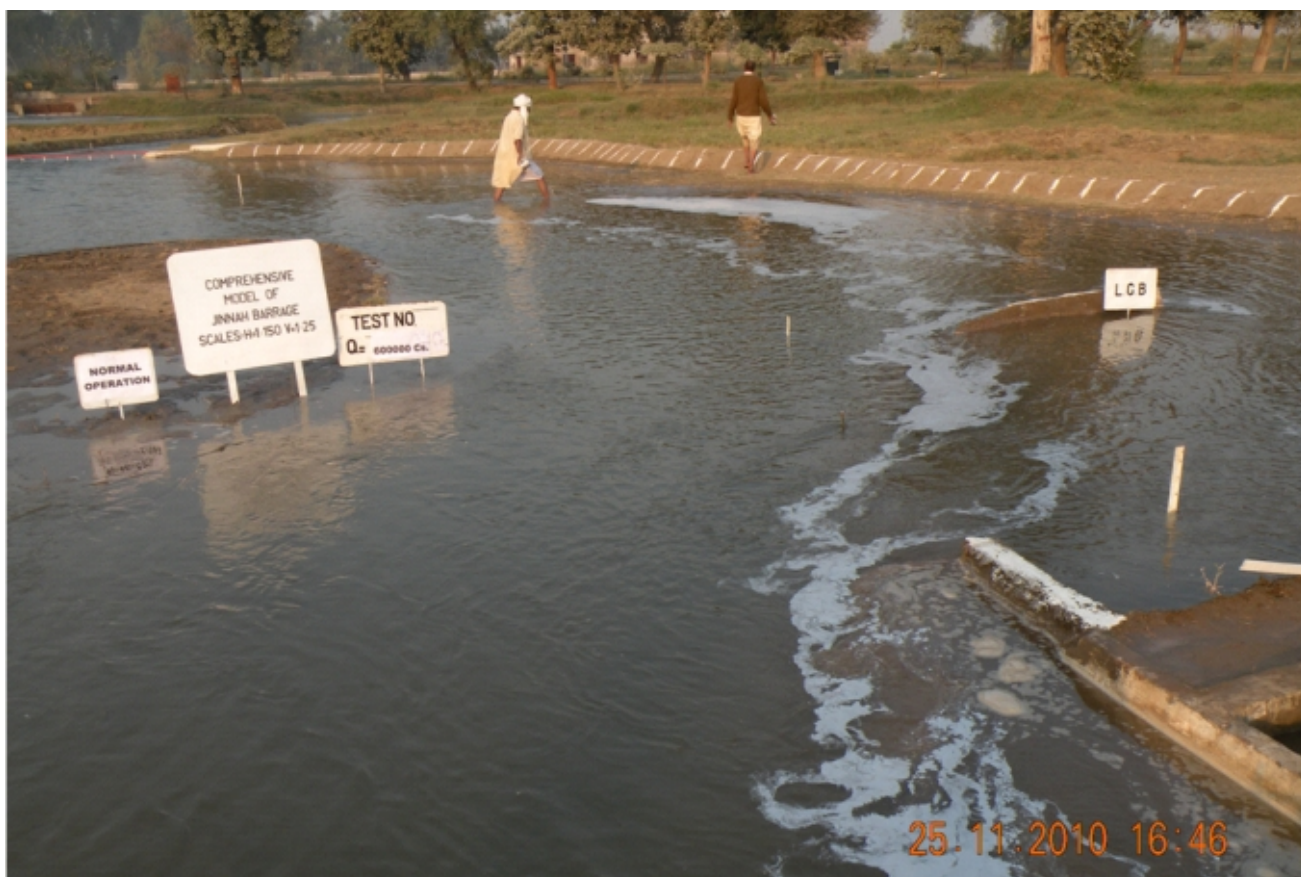
Normal Operation of Barrage at Q = 6,00,000 Cusec
