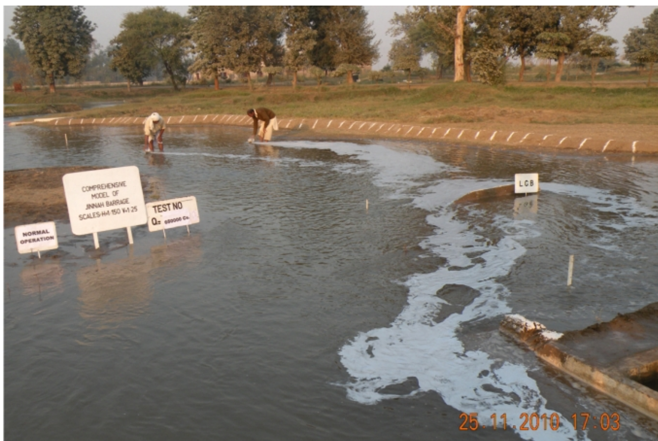
Normal Operation of Barrage at Q = 6,60,000 Cusec
